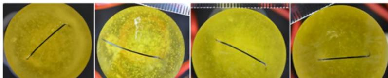
Fig.1. The four samples, embedded in acrylic VariDur 10 resin
